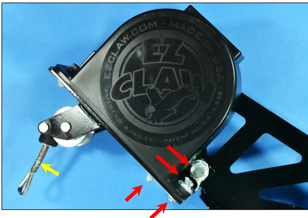
Figure 3: Closer view photograph of the EZ Claw retraction assembly after the completion of 120 hours of salt spray testing. No indication of red rust was visible. The white deposits (red arrows) around the fasteners are zinc oxide and are expected in zinc plated components. Additionally, an expected green copper oxide deposit (yellow arrow) was observed on the copper wire crimp. (Photo 2021104-N27)
