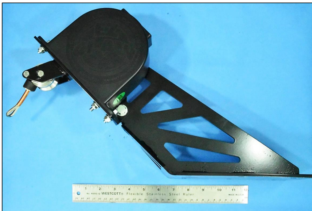
Figure 1: Photograph of the EZ Claw assembly prior to salt spray testing. The assembly was subjected to 120 hours of salt spray testing. (Photo 21104-N11)
