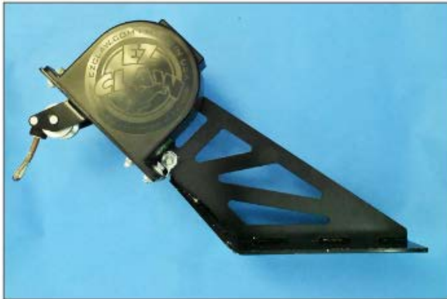
Figure 2: Photograph of the EZ Claw assembly after the completion of 120 hours of salt spray testing. No indication of red rust was visible. A closer view photograph of the retraction assembly is shown in Figure 3. (Photo 2021104-N26)
