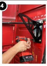
Mount the EZ Claw Truck Bracket using 5/16" flange bolts (included)
