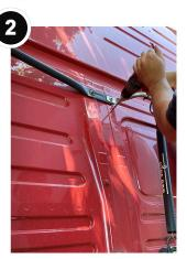
Using a 3/16" bit carefully drill pilot holes in the center of each mark (being careful not to plunge into insulation, wires etc.)
