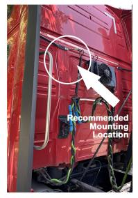
Select a mounting location vertically as high as possible to the left (driver's side) that will allow tying into a rib and without interference.
