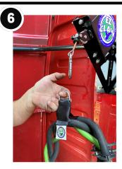
Using an EZ Claw Sling (sold separately) or other cable clamp, attach the EZ Claw tensioner cable to the hose and cable assembly.
