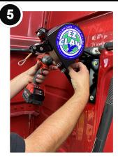
Mount the EZ Claw tensioner using the supplied 3/8" bolts and lock nuts.
