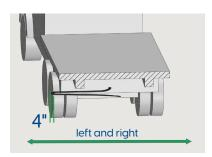
Connect lines to the rear of the truck. Pull the lines to the left and mark the point that is 4" past the mud flaps. Then, pull the lines to the right and mark the point that is 4" past the right mudflaps. If these marks are not in the same place, use the mark that is farthest from the truck.
