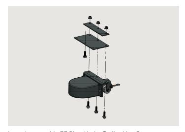
Loosely assemble EZ Claw Under Trailer Line Saver as shown above.
