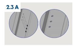
If using rivet nuts, install the provided rivet nuts in the holes with a rivet nut tool. Skip this step if you've tapped the holes and aren't using rivet nuts.
