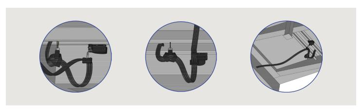
Connect the lines to the trailer. There should now be a loop in the lines between the trailer connections and the Hose & Cable Block. Use an EZ Claw Sling (included) to guide this portion of the lines to a safe location in front of the EZ Claw unit, where they won't rub or chafe on the Line Saver unit or crossmembers.
