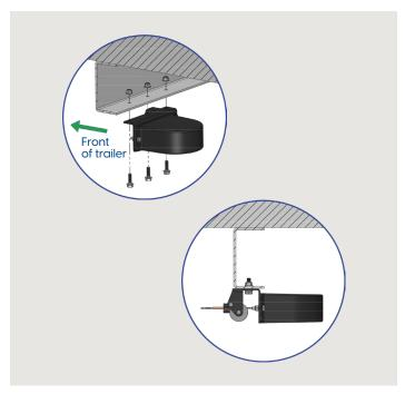
Mount the Line Saver onto the trailer with the provided nuts and bolts. Tighten all nuts with a 1/2" wrench and socket. Proceed to Step 3.
