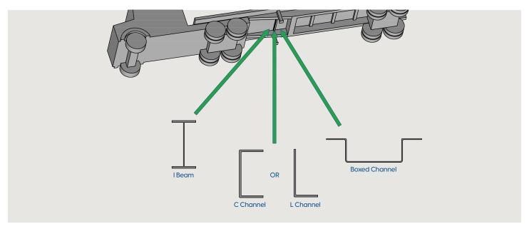
Determine the shape of the crossmember the EZ Claw Line Saver will be mounted to. Proceed to the corresponding Step 2 for your crossmember shape.
