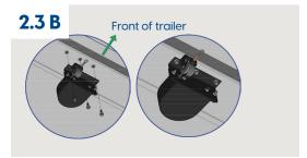
Hook the Delta Quicklink on the Hose & Cable Block onto the loop on the end of the line saver cable. Tighten the nut on the Delta Quicklink with a wrench to prevent loosening.
