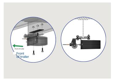
Hook the assembly onto the I-beam, centering it between the landing gear. Install the remaining bolts, nuts and plate onto the Line Saver. Tighten all nuts with a 1/2" wrench and socket. Proceed to Step 3.
