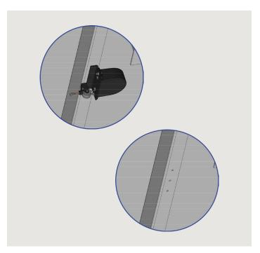
Hold the Line Saver up to the center of the crossmember between the landing gear. Trace the three holes in the bracket onto the crossmember and then drill them out with a 3/8" drill bit.
