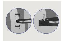
Install the Hose & Cable Block at the mark you made above.
