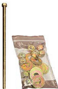
MOUNTING HARDWARE (QTY 8) 1/2-13 x 13" LONG G8 BOLT (QTY 16) 1/2-13 G8 FLAT WASHER-YZN (QTY 8) 1/2-13 G8 LOCK NUT-YZN
