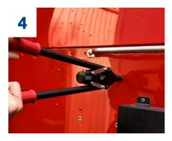
**Install Rivet Nuts.**
