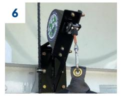
**Install Line Saver.** Mount the EZ Claw Line Saver utilizing the 3/8" mounting hardware supplied with the Line Saver.
