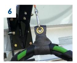
Attach Hose Assembly. Using an EZ Claw Sling (EZCS) or Hose & Cable Block (EZCHCH38), attach the EZ Claw Line Saver cable to the hose assembly.
