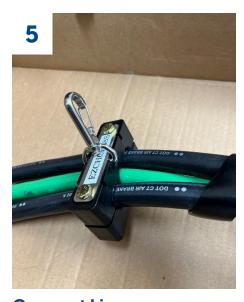
**Connect Lines.** Install 3-in-1 wrapped air and electric lines. Cut the spiral wrap in the approximate center of the of the lines and install the Hose & Cable Block (EZCHCH38) on hoses.
