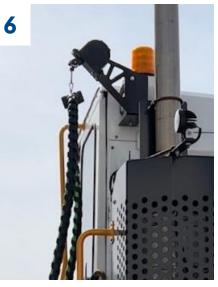
Attach Hose Assembly. Using an EZ Claw Sling (EZCS) or Hose & Cable Block, attach the EZ Claw Line Saver cable to the hose assembly.
