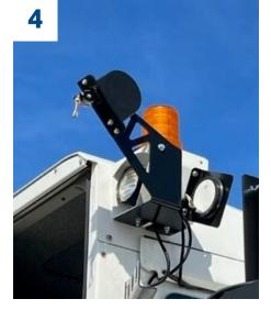
**Tighten Bracket.** Install EZ Claw Yard Truck Line Saver on Yard Truck Adapter bracket utilizing supplied 3/8" hardware.
