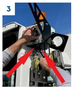
**Spotlight Options.** Install additional supplied 5/16" hardware (bolt/washers/lock nut) in bottom two holes indicated by the red arrows above. If rear-facing spotlight was removed in Step 1, utilize the stud from the spotlight instead of the bolt supplied and re-install the spotlight.
